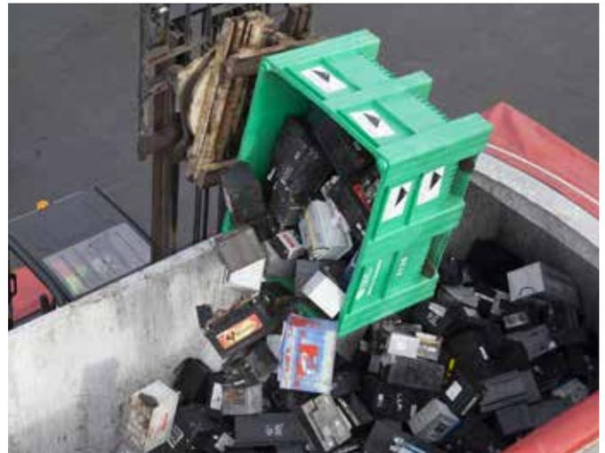
Tipping lead-acid batteries into trailer for smelting
